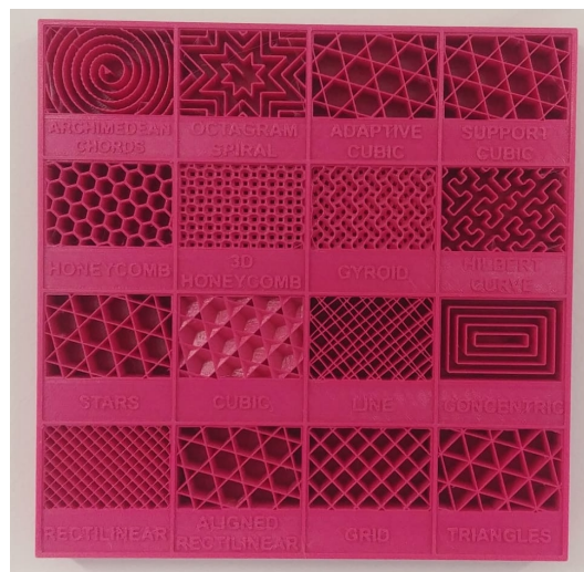
Figure 12: Types of possible profiles to use as infill. This model is exposed at SKIL (EPFL) [45]
