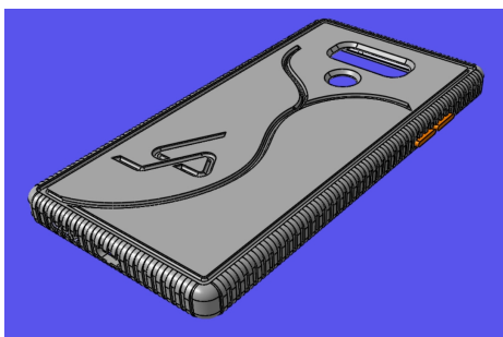
Figure 30: Rendering of the front and back of the second phone cover. Notice the fact that the volume buttons have been added as a separate component (orange part)
