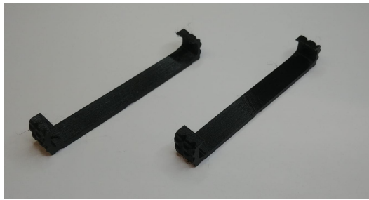
Figure 28: Test parts, printed each with different tolerances (-0.2mm and -0.4mm), in order to check which one fits best around the phone
