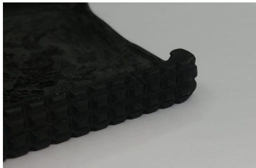
Figure 29: Crack on the phone cover. Notice how the crack continues between two layers (weak spot)
