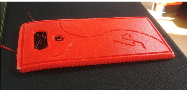
Figure 35: Left image: unfinished cover, Right image: finished cover, even though the corners got detached from the bed
