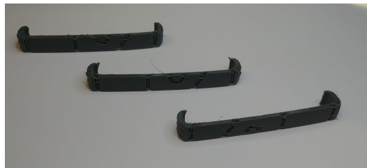
Figure 32: Test parts replicating the width of the phone cover. The three parts are bigger than the original by 0.2, 0.4 and 0.6mm
