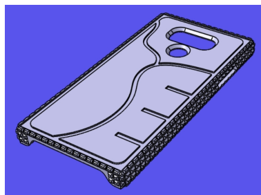
Figure 25: First design for the cover. The planned material of print is PETG
