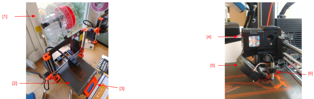
Figure 3: Images of Prusa MK3S model FDM 3d printer [58]
