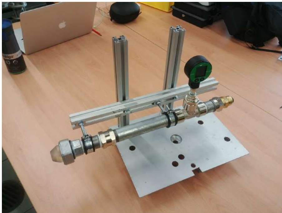
Figure 10: Support for the wind tunnel. The support is very rudimental. Still, it allows regulation of height due to the sliding grooves on the profile
