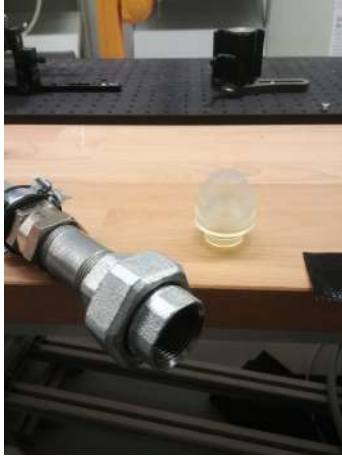
Figure 9: On the left image, the fixation (commonly used in plumbing) is shown. One element of the fixation was redesigned to be the nozzle, leading to the design on the right
