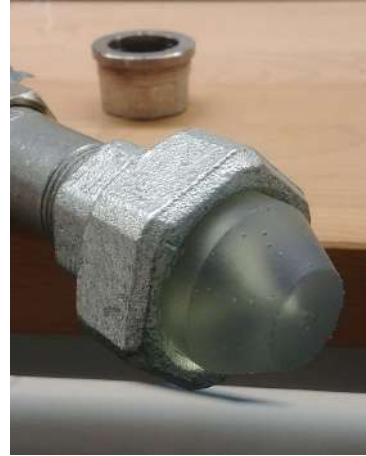
Figure 9: On the left image, the fixation (commonly used in plumbing) is shown. One element of the fixation was redesigned to be the nozzle, leading to the design on the right
