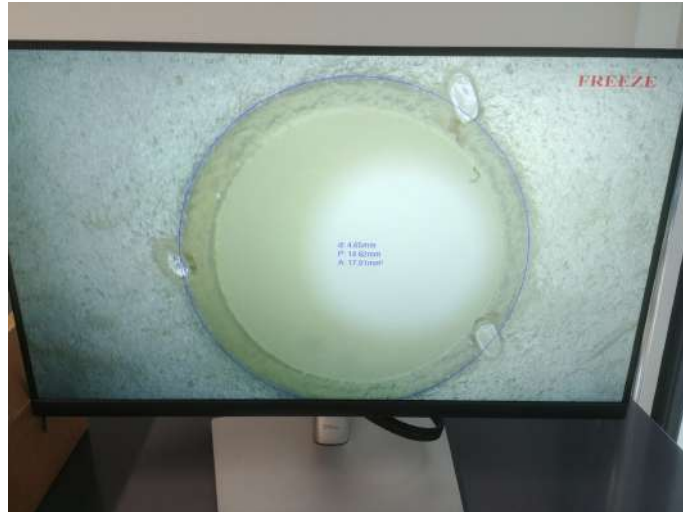
Figure 33: Closeup view of Nozzle_V0, showing the presence of three support pins. Those pins were placed close to the nozzle on the Formlabs slicer, however they were found to be in the way of the nozzle exit on the real nozzle.
